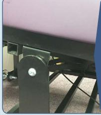
The arms are removable and / or adjustable for seat width. Each arm is supported on two square tubes which slide within two other square tubes.
