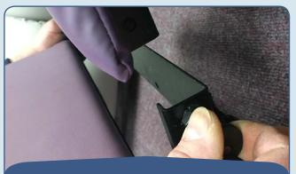
Footplate removal requires two hands to pull each of the index plungers out and then slide the footplate off the leg rest mechanism.
